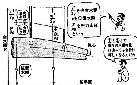
$$\frac{v_1^2}{2g} + z_1 + \frac{p_1}{\rho g} = \frac{v_2^2}{2g} + z_2 + \frac{p_2}{\rho g} = E$$
