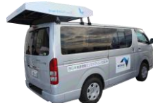
舗装三要素の簡易計測 (Smart-EAGLE type-P)
