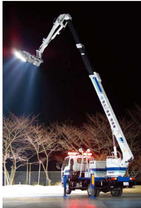
照明車(2kW×6灯)
