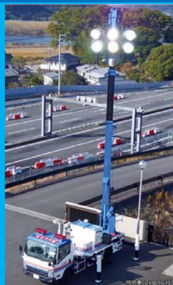
照明車(2kW×6灯)
