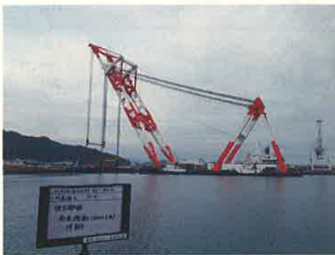
大型起重機船(4,000t吊)
